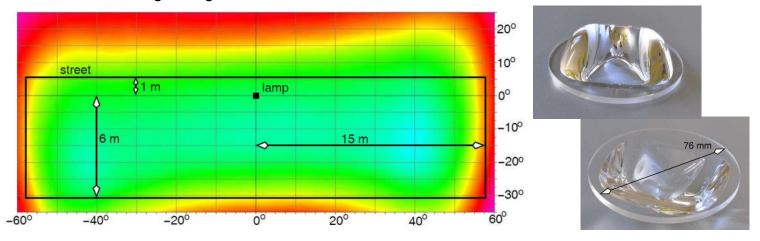
Lens is designed for high power LEDs (over 30 W) with size from 12x12mm to 18x18mm. One lens is used per one LED. Measured lighting angle is 45x110° which corresponds to illuminated area 8.5x30m when lamp is 10m above the ground.
